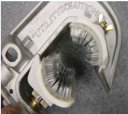
CLOSE UP VIEW SHOWING AGGRESSIVE WIRE BRUSHES AND EASY REMOVAL SYSTEM
