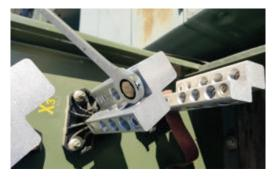
The low profile design allows access to connectors when space is limited. Just 1/2" is exposed above the bar, while a 1/2" allen driver fully engages the connector to avoid stripping. Low profile means less chance of touching other connections or exposed metal.
