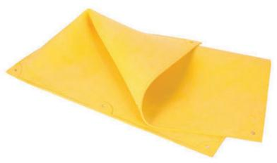
Utility Solutions Insulated Rubber Blankets are Type II, Style "A" and manufactured from EPDM to provide maximum resistance to ozone damage. They are molded in high visibility yellow and are free from any internal reinforcement for maximum flexibility.
