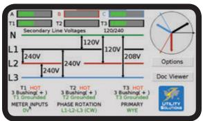
secondary, modify phase orientation. explore multiple secondary voltages and different transformer settings. simulates back-feeding and reduced capacity services so users learn and practice real-world troubleshooting.
