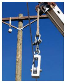
Unlike imported cast blocks, the Conductor Lift Snatch Block is USA made and machined from solid aluminum. The compact design offers a 1500 pound m a x i m u ml working load yet weighs only 3 lbs.
