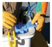
drainage holes in the base provide rain drainage to ensure the interior stays dry. The cover/base design permits bucket stick storage without the need to rotate the hot stick probe end and permits one to grab the stick body when removing so as not to extend the stick.
