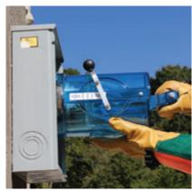
Molded of a rugged polymer the tool is rugged, lightweight and tinted to allow the operator to visually observe the entire operation.
